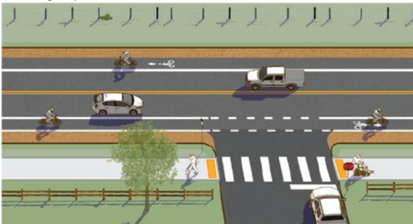
A typical complete street solution for more populous areas would be to accommodate bicycle lanes on either side of the road, and a sidewalk on at least one side of the road. - Photo Credit: Federal Highway Administration
