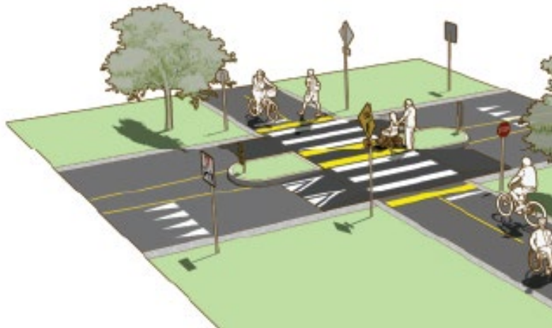
A shared use path constructed parallel to and within the right-of-way. Photo Credit: Federal Highway Administration
