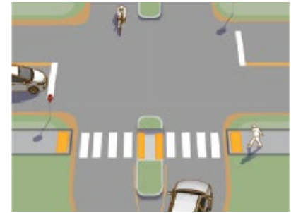
Median Island – Photo Credit: Federal Highway Administration
