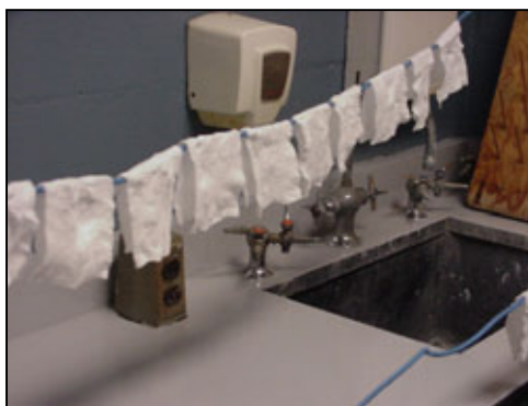
Figure F4.3: Drying the Pads
